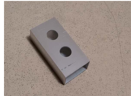
Fig. 1. Cutting of holes in aluminum alloy of 2mm width
