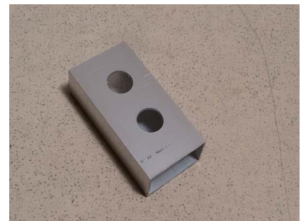
Fig. 1. Cutting of holes with diameter of 15mm in aluminum alloy of 2mm width
